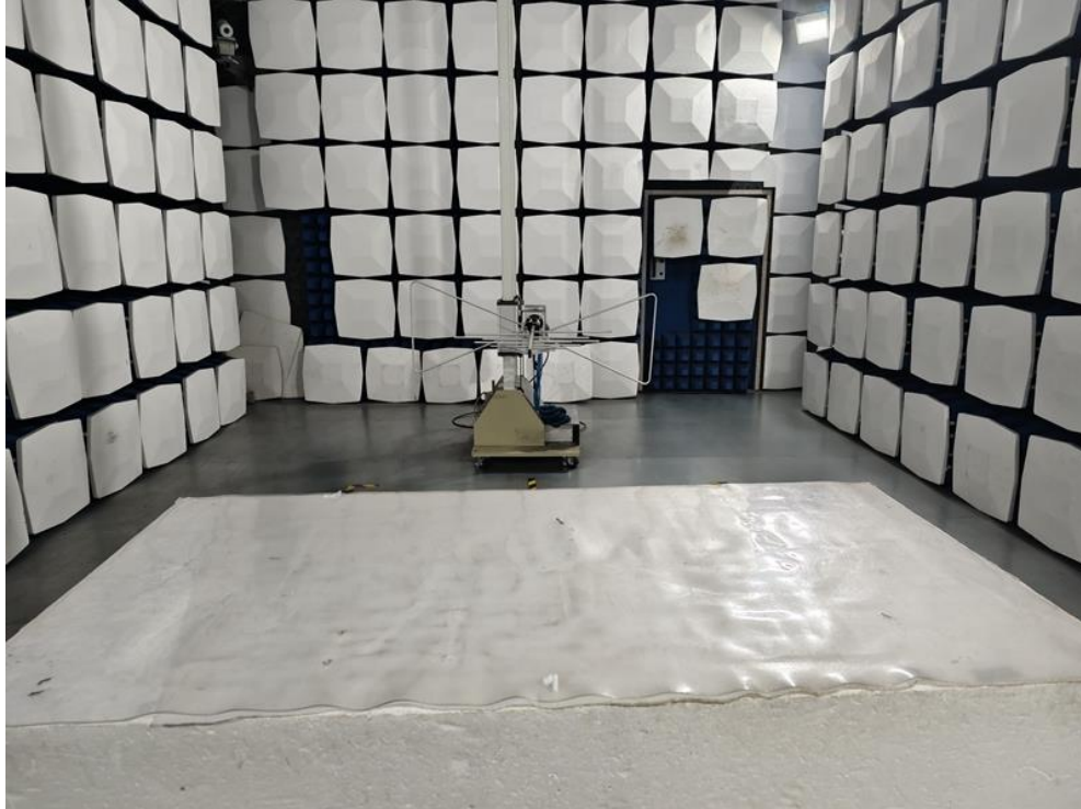
Radiated Emission Test Setup:
