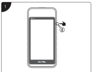
• Long press the **Power/Lock** button to turn on the tool.
