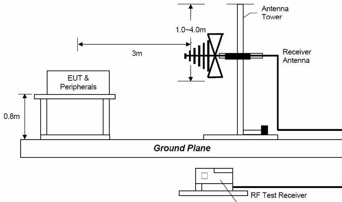
Radiated Emission Test Set-Up, Frequency above 1GHz
