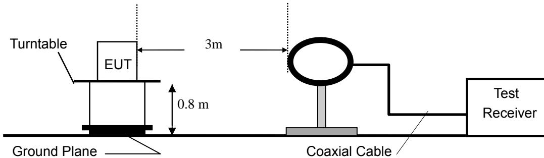
Radiated Emission Test Set-Up, Frequency Below 1GHz
