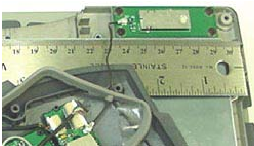
Distance between external dipole antenna feed/swivel-joint and internal Bluetooth surface-mount antenna
