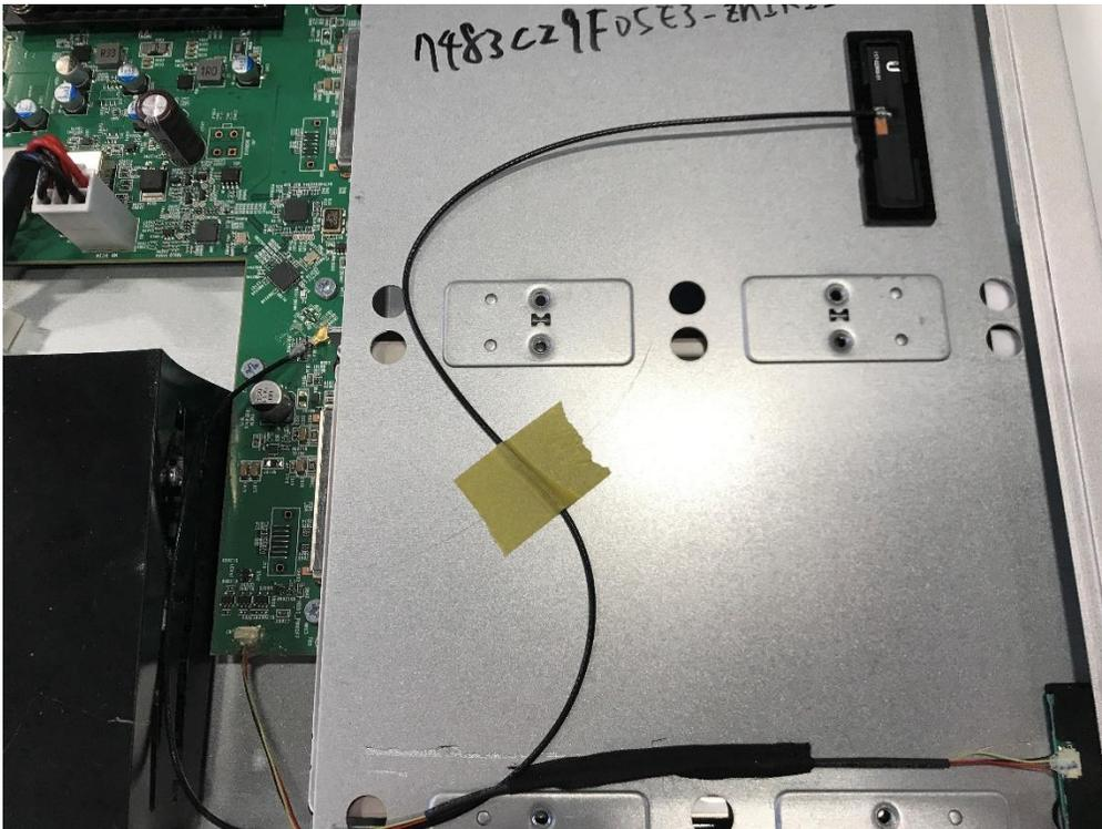
**Photograph 2: Antenna of Bluetooth Transmitter**
