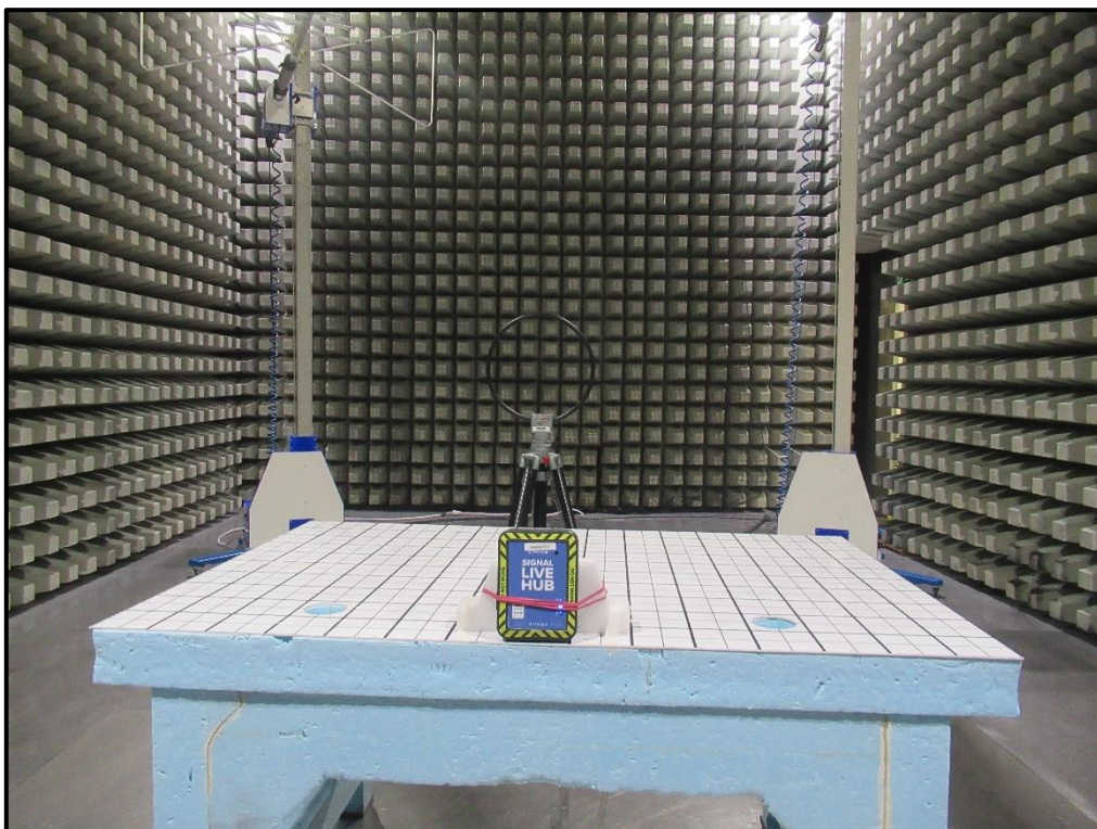
Photo 2 Radiated Test Setup from 9 kHz to 30 MHz
