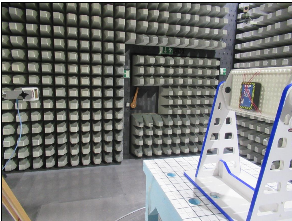
Photo 8 Radiated Test Setup from 18 GHz to 25 GHz
