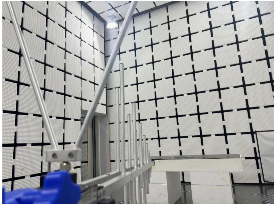
Radiation Emission Test Setup (30MHz to 1GHz)
