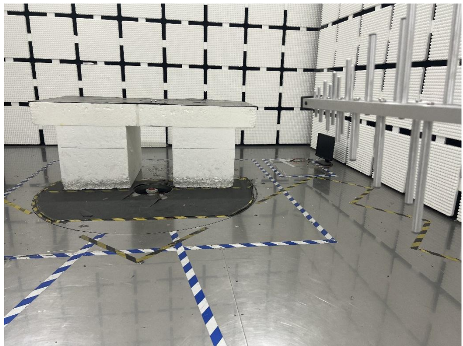
Radiation Emission Test Setup (30MHz to 1GHz)
