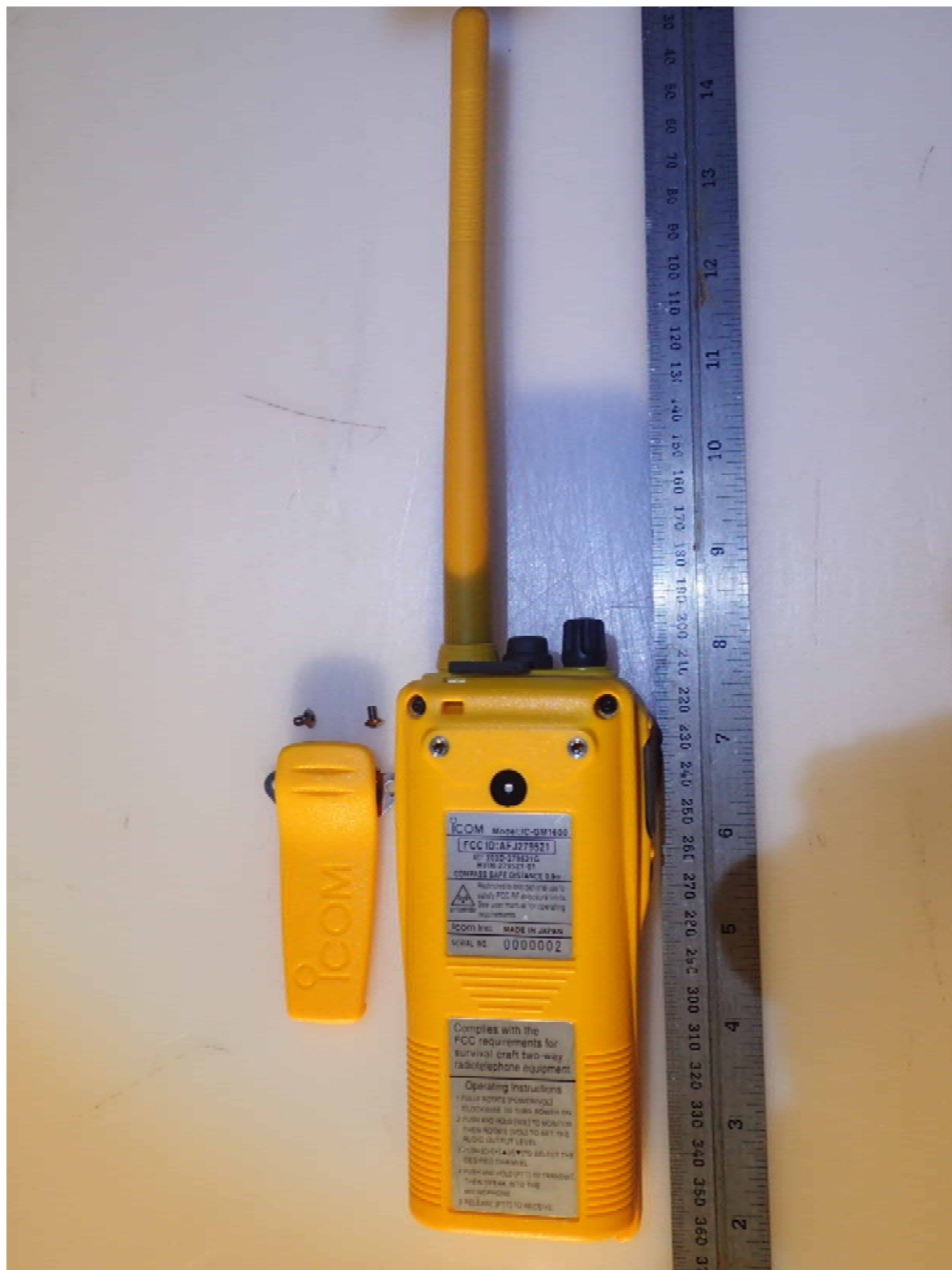
< D.U.T.'s rear view without battery and MB-103Y Belt Clip removed >
