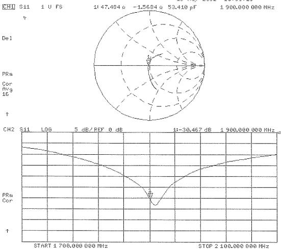
Validation Dipole D1900V2 SN504, d = 10 mm
