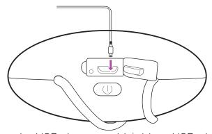
2. Insert the USB charging cable's Micro USB plug into the charging port on your speakers.
