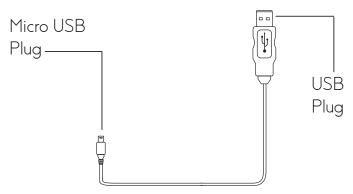
1. The USB charging cable has a Micro USB plug and a standard USB plug.
