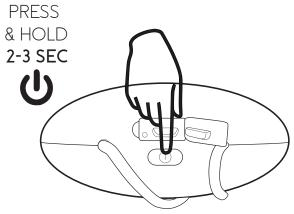
1. Press and hold the power button for 2-3 seconds to power on your speaker. If it has been previously paired to your Bluetooth device. it will automatically remain paired each time it is powered on.
