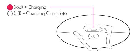
4. The LED Indicator Light turns red while the speaker is charging then turns off once charging is complete.
