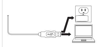
3. Insert the USB charging cable's standard USB plug into the USB port of a computer or suitable USB charging adapter.
