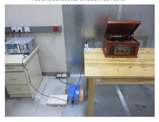
FCC RADIATED EMISSION TEST SETUP
