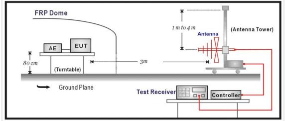
1GHz -40GHz Test Setup:
