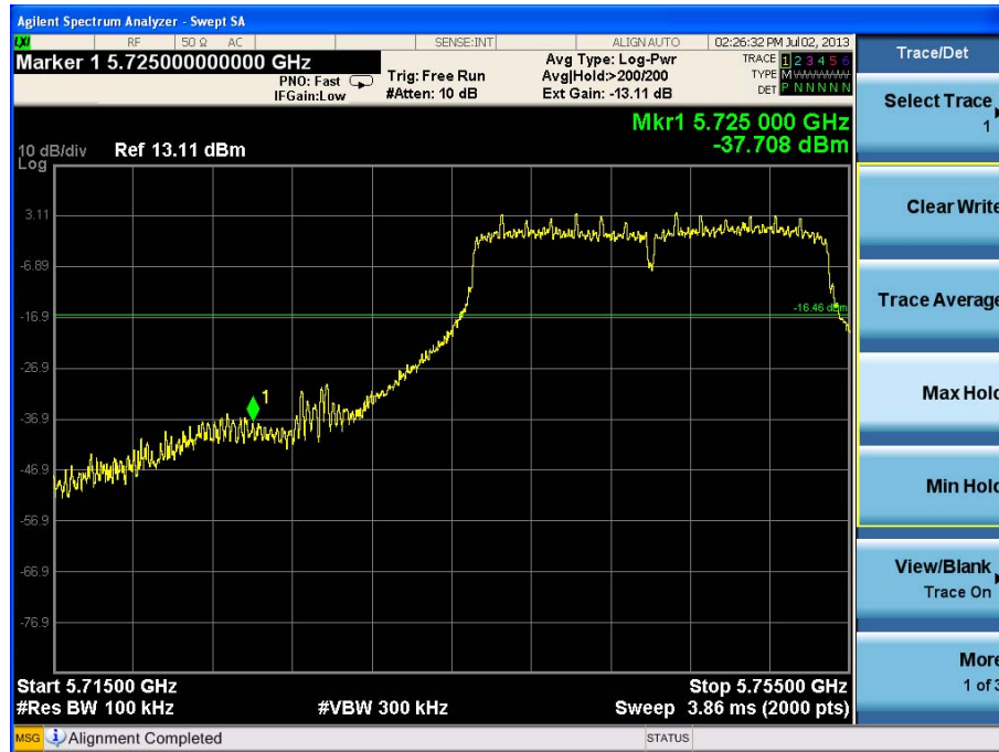
Figure 4.7.1 The Worst Peak Out-of-Band Emissions Near Band Edge for 20MHz Carriers, 802.11n (20MHz-2Tx-1S) Carrier at Channel 149/5745MHz, 18dBm Setting (both Medium Gain and High Gain Antenna), OFDM/CDD, MCS0, Port 1.
