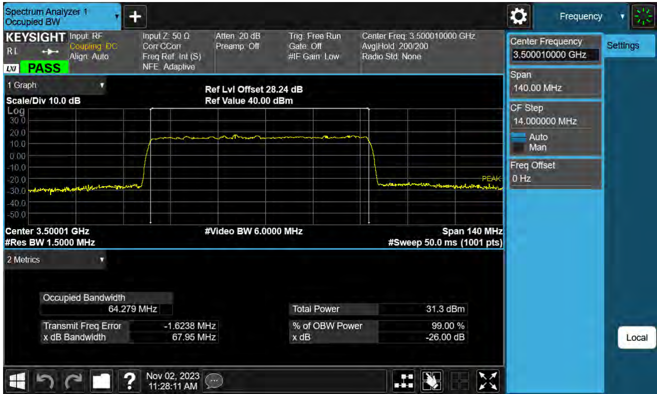
Sub6 n77(78). Occupied Bandwidth Plot (70 M BW Ch.633334 QPSK )
