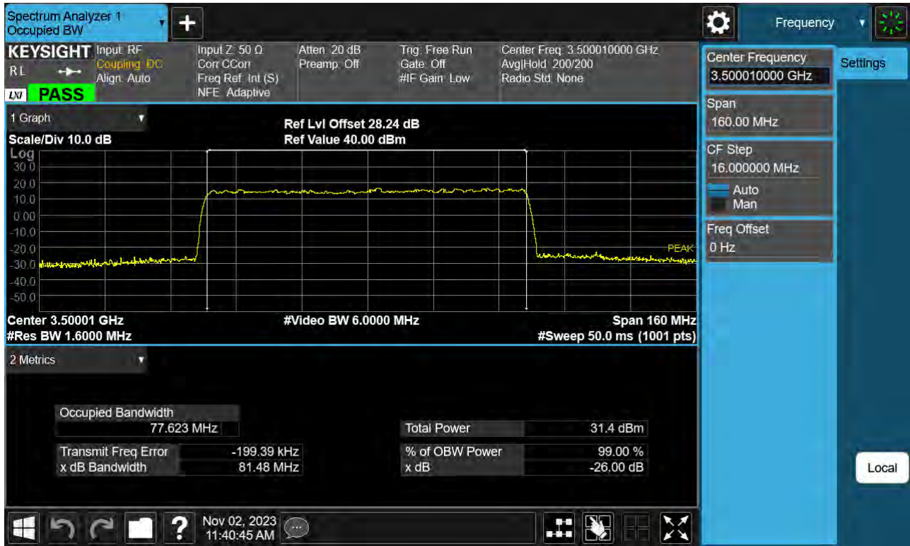
Sub6 n77(78). Occupied Bandwidth Plot (80 M BW Ch.633334 QPSK )
