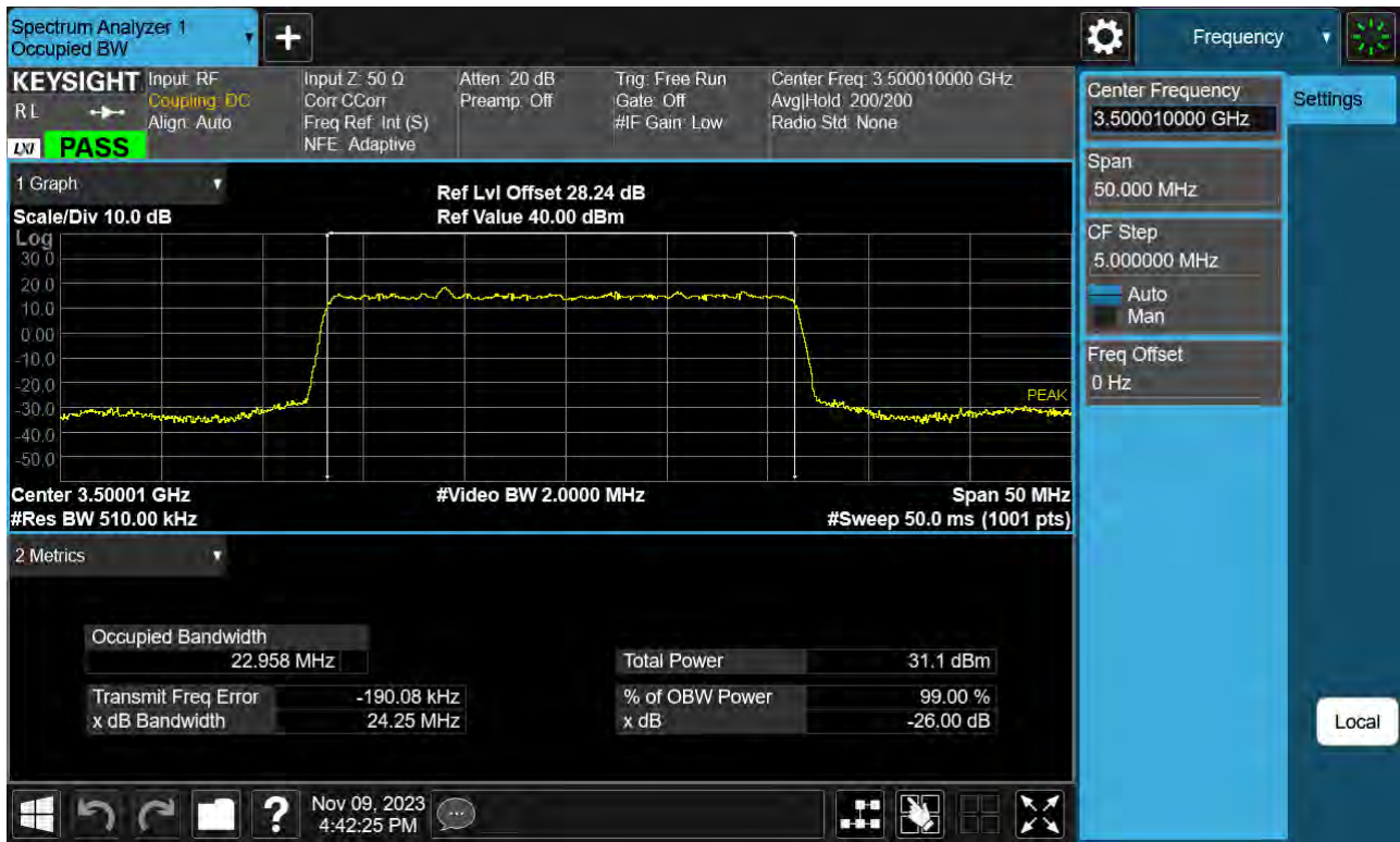
Sub6 n77(78). Occupied Bandwidth Plot (25 M BW Ch.633334 BPSK )
