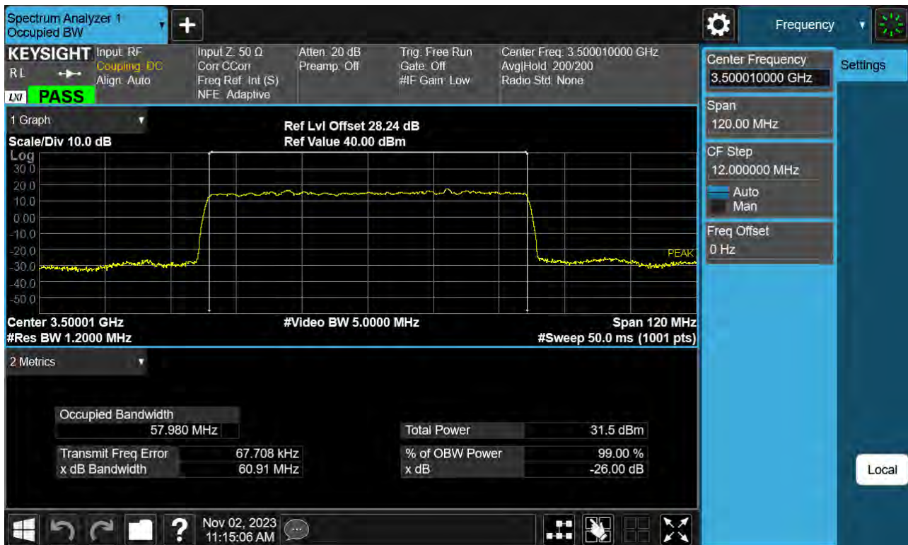
Sub6 n77(78). Occupied Bandwidth Plot (60 M BW Ch.633334 BPSK )
