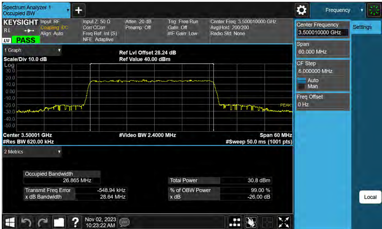
Sub6 n77(78). Occupied Bandwidth Plot (30 M BW Ch.633334 QPSK )
