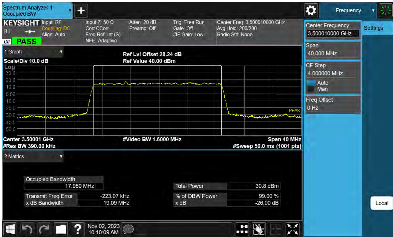
Sub6 n77(78). Occupied Bandwidth Plot (20 M BW Ch.633334 BPSK )
