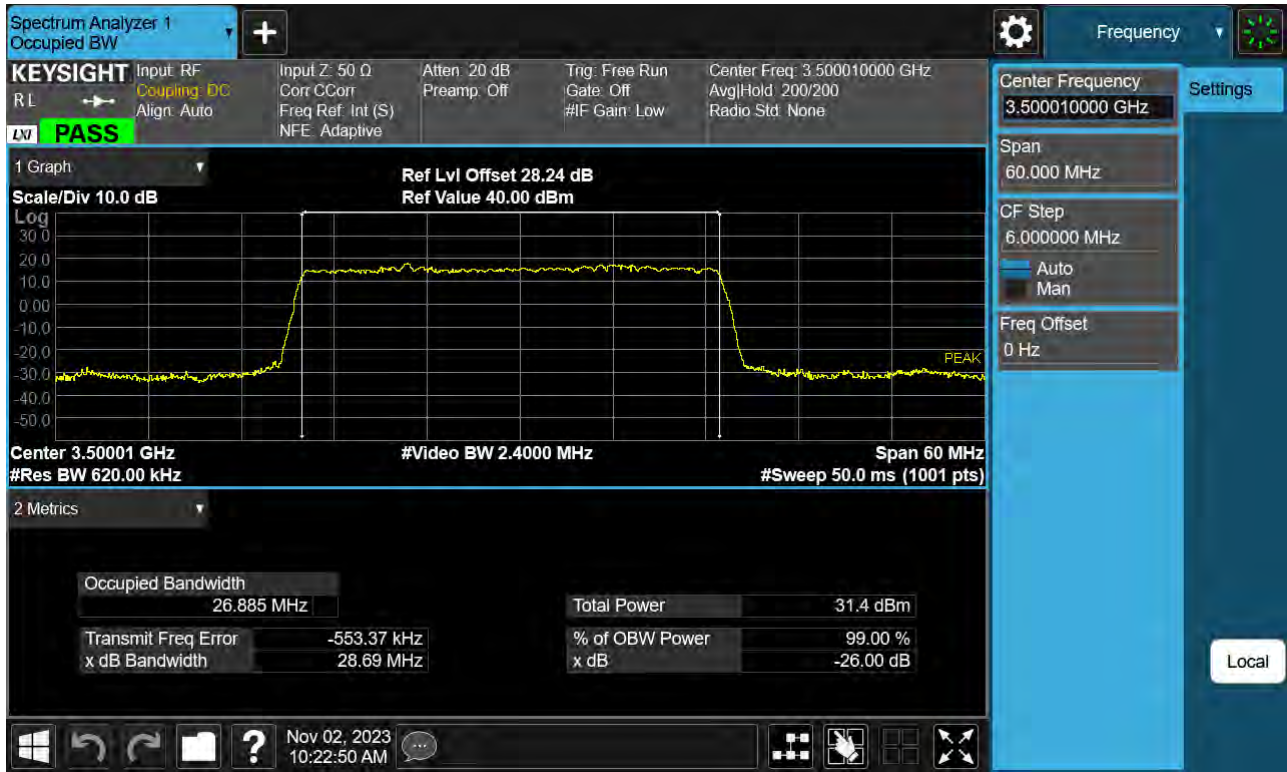
Sub6 n77(78). Occupied Bandwidth Plot (30 M BW Ch.633334 BPSK )
