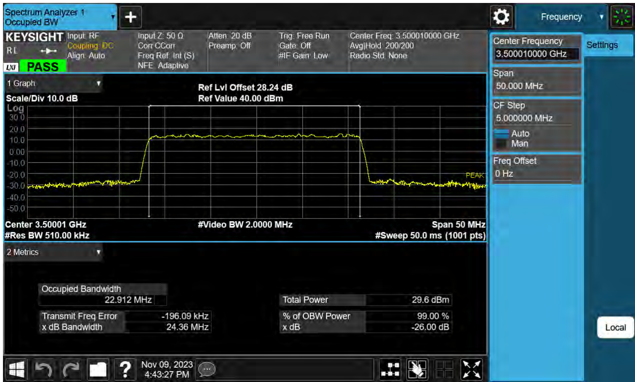
Sub6 n77(78). Occupied Bandwidth Plot (25 M BW Ch.633334 16QAM )
