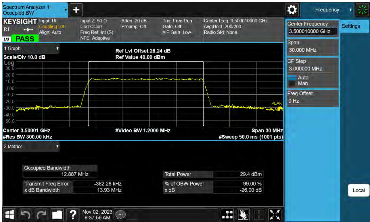
Sub6 n77(78). Occupied Bandwidth Plot (15 M BW Ch.633334 16QAM )
