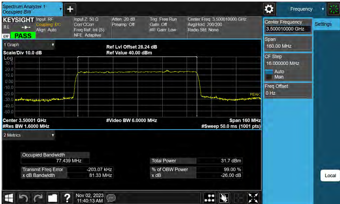
Sub6 n77(78). Occupied Bandwidth Plot (80 M BW Ch.633334 BPSK )
