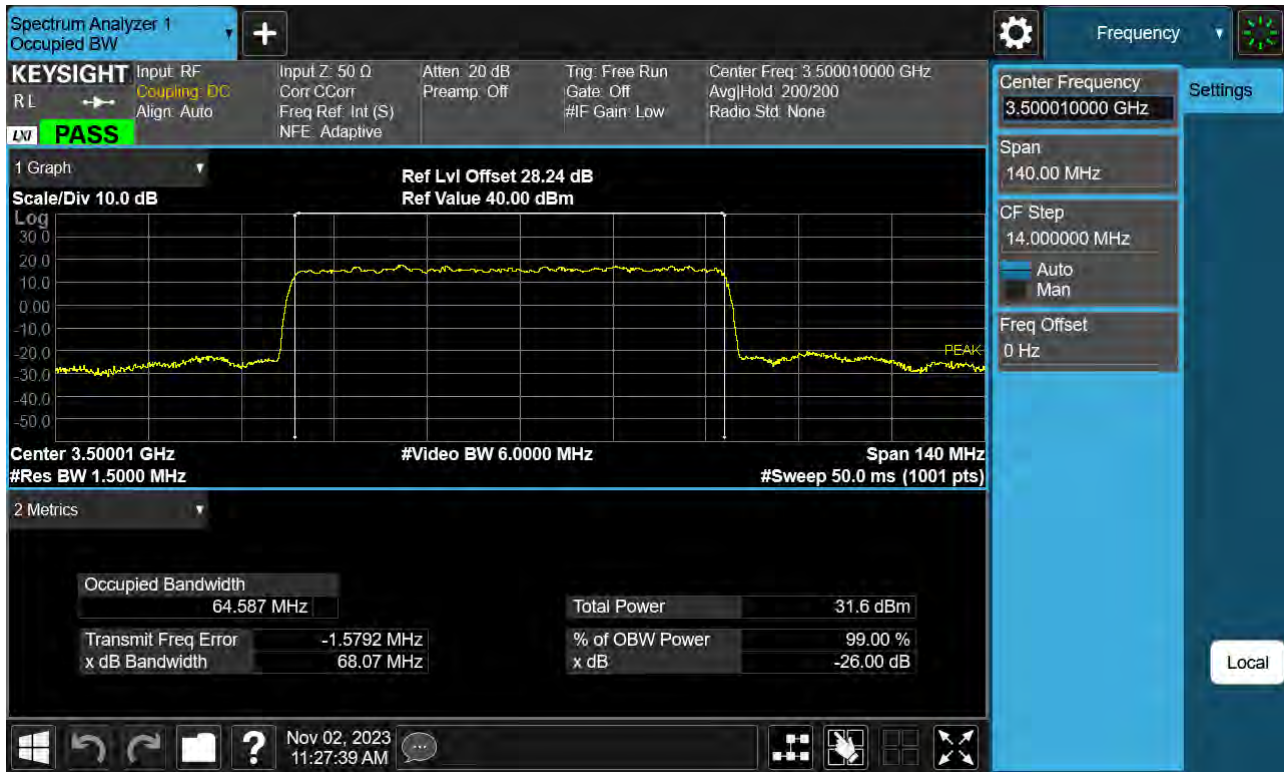
Sub6 n77(78). Occupied Bandwidth Plot (70 M BW Ch.633334 BPSK )
