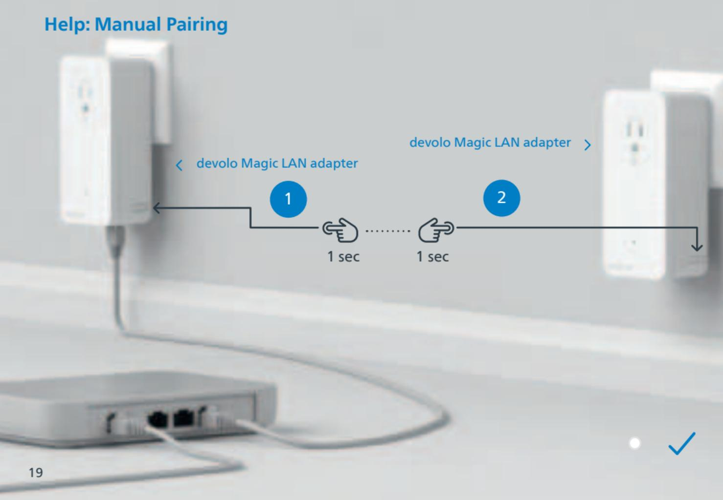
**| GB |** Within 3 minutes, press the button on the side of your devolo Magic LAN adapter, which is connected to the router. Then press the button on your second Magic LAN adapter. When all of the LEDs light up white, pairing has been completed successfully.
