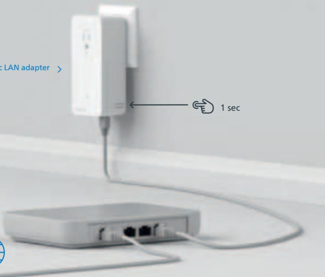
**| US |** Within 3 minutes, press the button on the side of your devolo Magic LAN adapter which is connected to the router.
