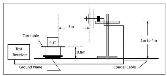
(c) For radiated emissions above 1000MHz
