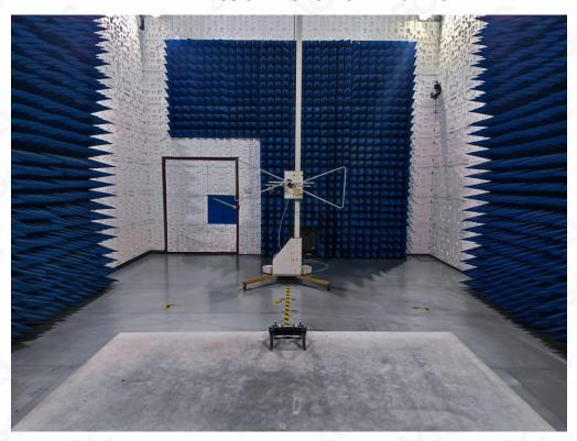
RADIATED EMISSION TEST SETUP ABOVE 1GHz
