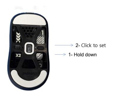
Gather Step 1: Hold the "Hz" switch and click the DPI button to switch Debounce Time. At this time, OLED will only display the current set value, other set values will be hidden; Gather Step 2: After the setting is complete, wait 1 second, OLED will return to the main i nterface:
