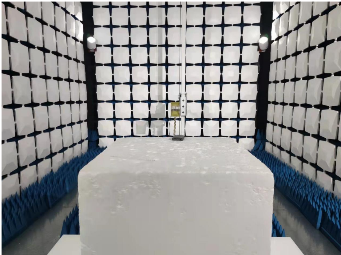
Above 1GHz for radiated emission test setup
