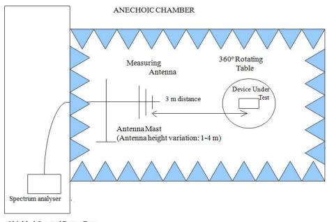
Shielded Control Room For Radiated Measurements
