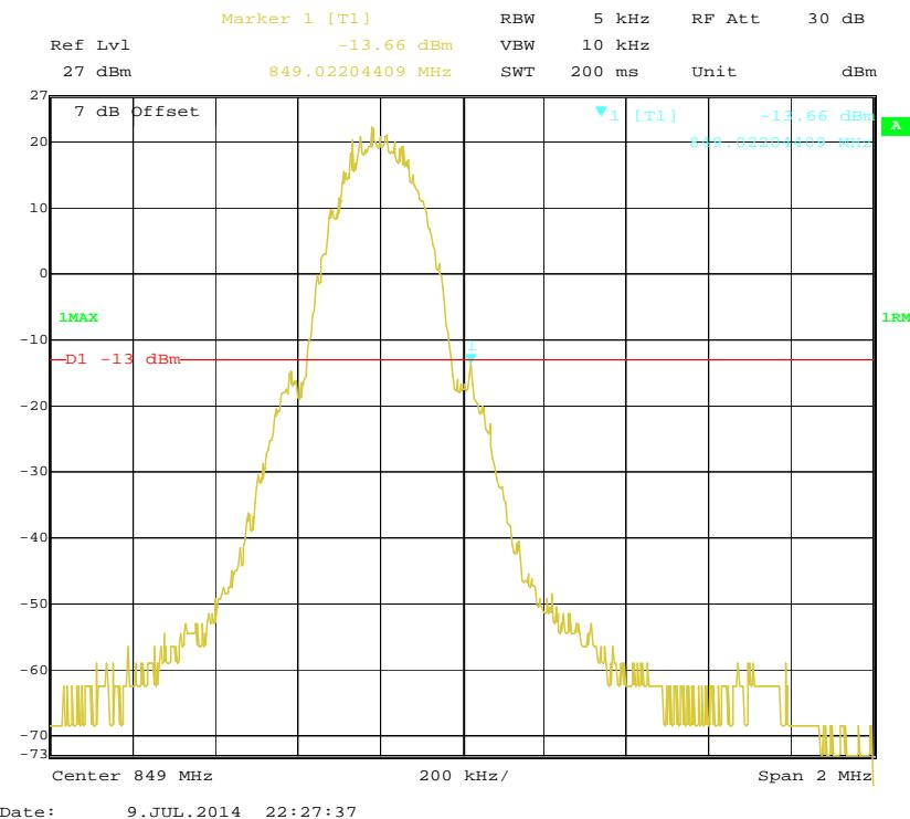
**Cellular Band, Left Band Edge for EDGE (8PSK) Mode**
