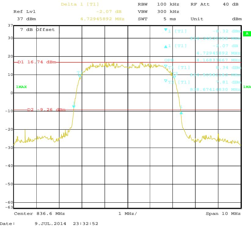
**PCS Band (Part 24E)****99% Occupied & 26 dB Emissions Bandwidth for GSM (GMSK) Mode**
