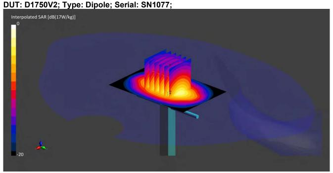
Communication System: CW UID: 0; Frequency: 1750.0 MHz; Duty Cycle: 1;
