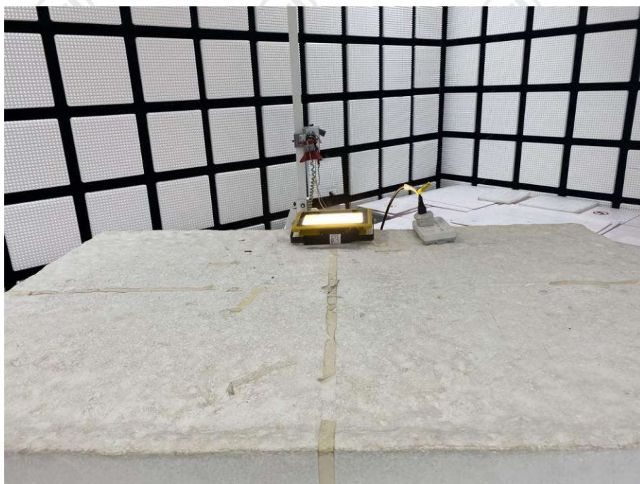
Radiated spurious emission Test Setup-2(Above 1GHz)
