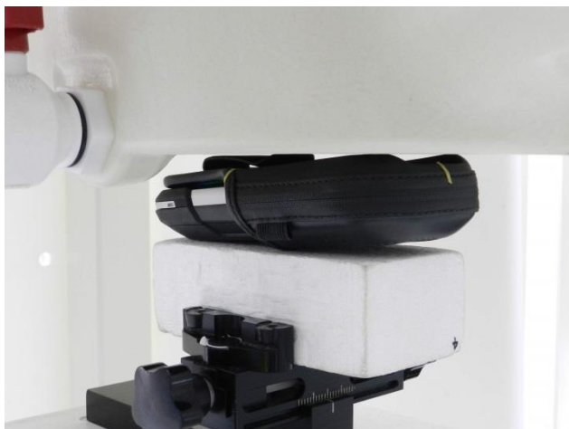
Front with soft holster, Test Separation 0 mm
