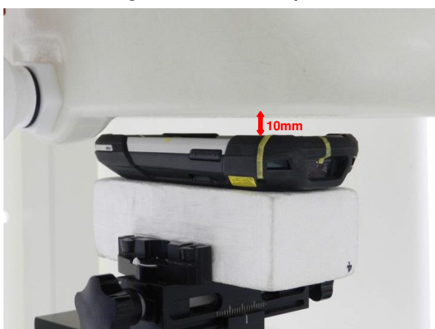
Front, Test Separation 10 mm
