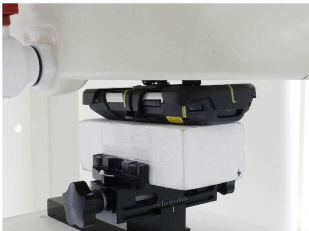
Front with rigid holster, Test Separation 0 mm
