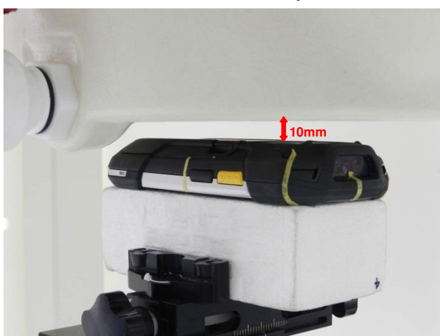
Back, Test Separation 10 mm
