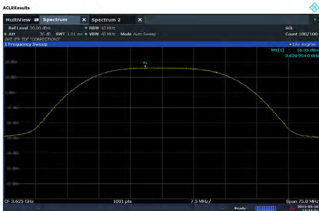
Plot 7.90. Conducted Power / 10MHz (30MHz 16QAM, Mid Channel – Ch.B)
