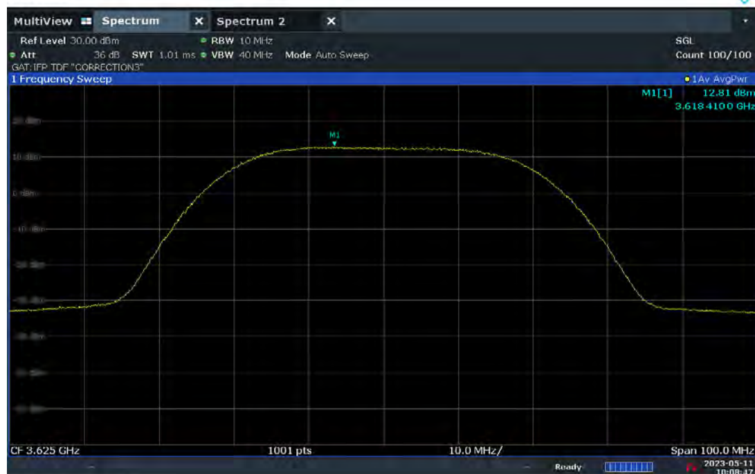
Plot 7.80. Conducted Power / 10MHz (40MHz 256QAM, Mid Channel – Ch.A)
