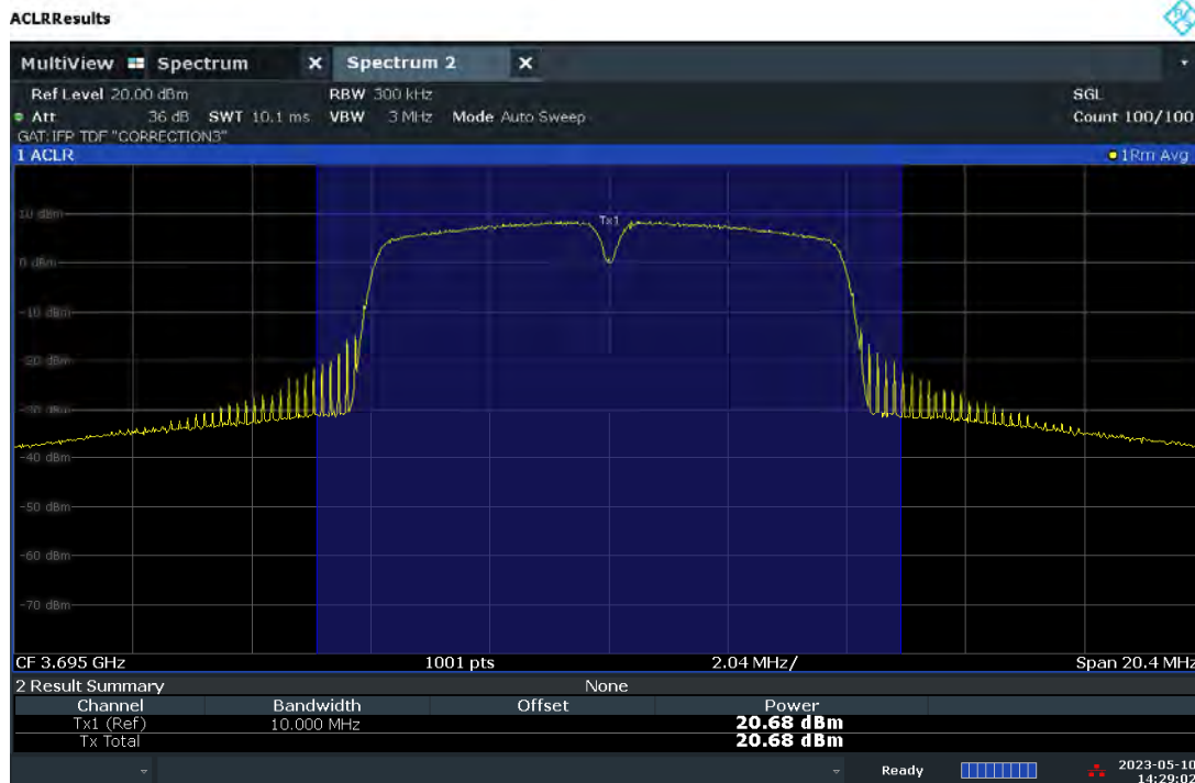
Plot 7.19 – Conducted Power Measurement – 10MHz BW, High Channel, 64QAM – Ch.B
