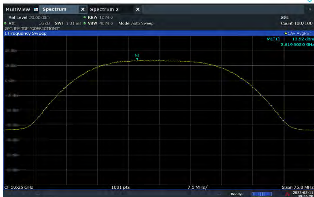
Plot 7.76. Conducted Power / 10MHz (30MHz 256QAM, Mid Channel – Ch.A)
