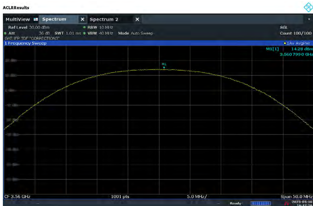
Plot 7.70. Conducted Power / 10MHz (20MHz 16QAM, Low Channel – Ch.A)
