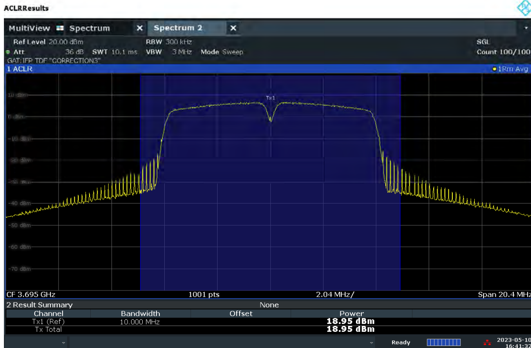
Plot 7.3 – Conducted Power Measurement – 10MHz BW, High Channel, 64QAM – Ch.A
