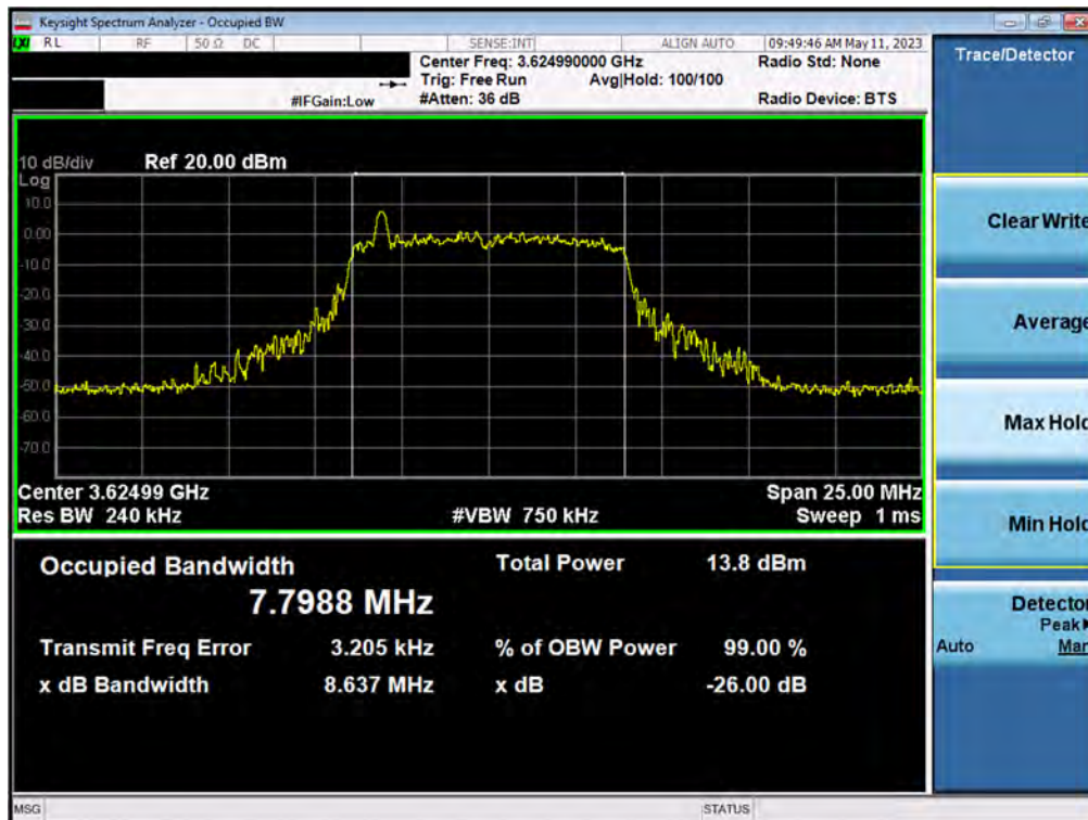
Plot 7.48. Occupied Bandwidth Plot (10MHz 256-QAM – Ch.A)
