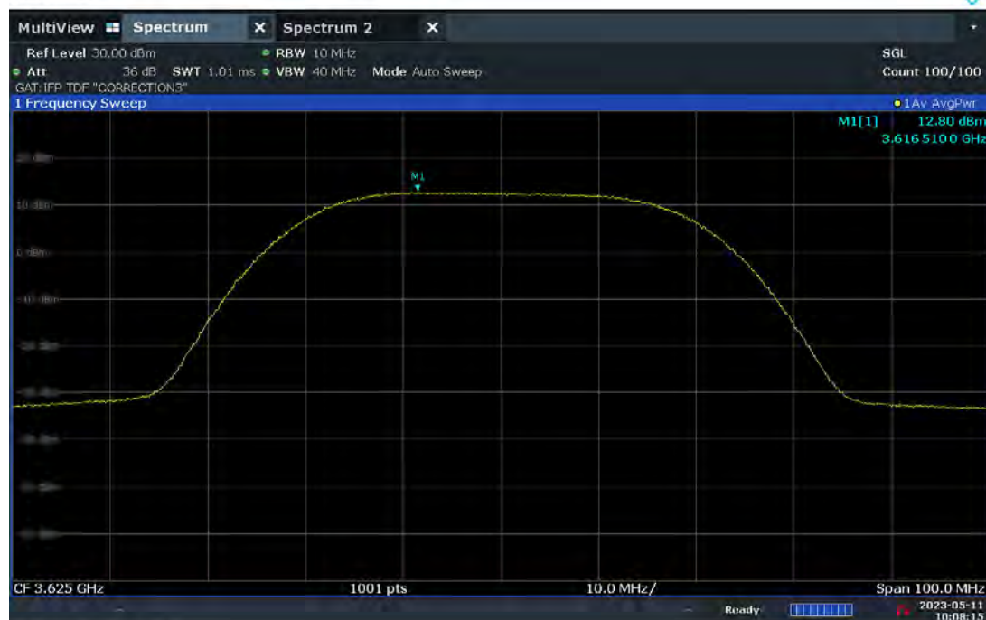
Plot 7.79. Conducted Power / 10MHz (40MHz 64QAM, Mid Channel – Ch.A)
