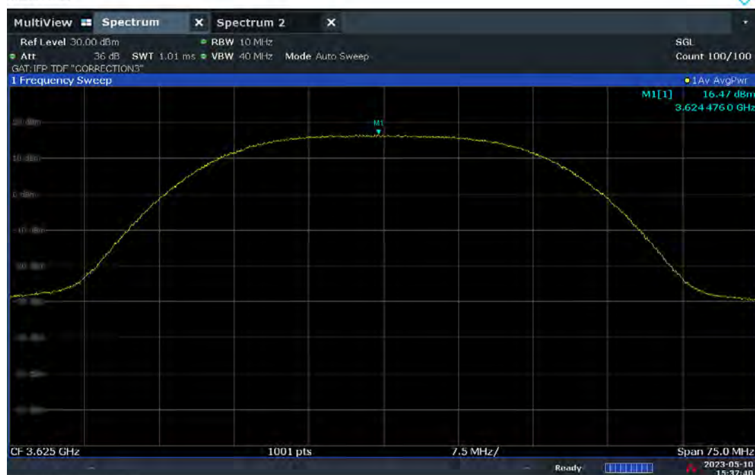
Plot 7.92. Conducted Power / 10MHz (30MHz 256QAM, Mid Channel – Ch.B)
