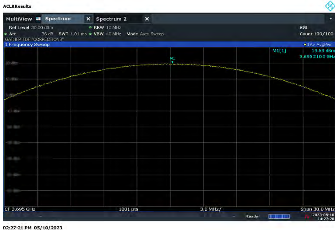
Plot 7.81. Conducted Power / 10MHz (10MHz QPSK, High Channel – Ch.B)
