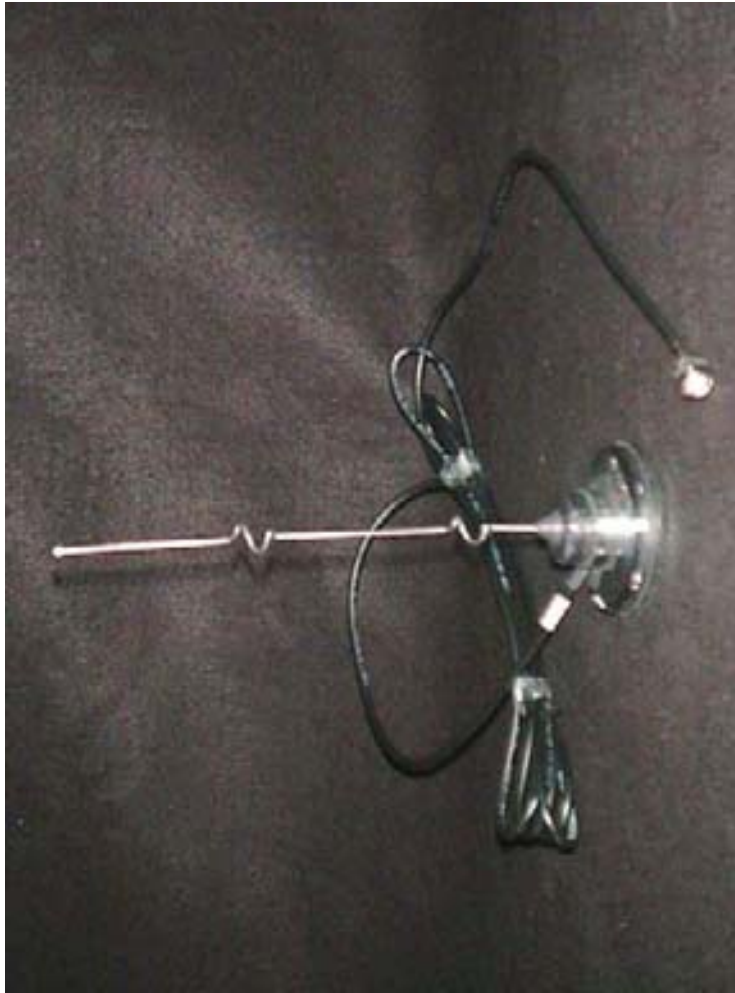
Photo 3. Antenna, MaxRad 5 dBi Whip (M/N MUF24005-RTNC)
