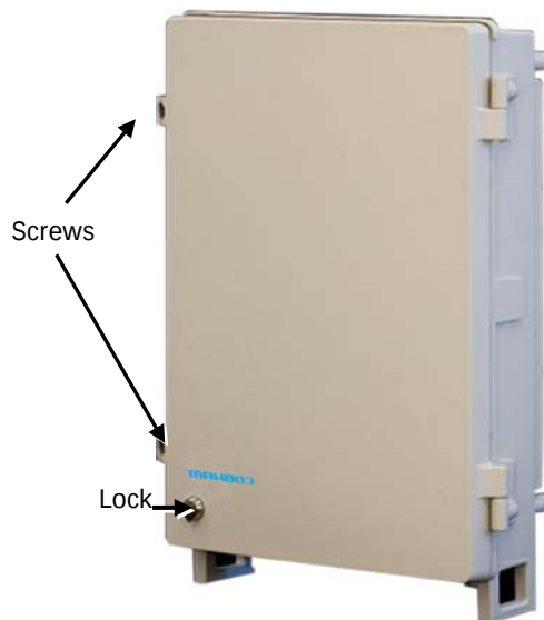
Figure 2-32: Securing the Repeater
