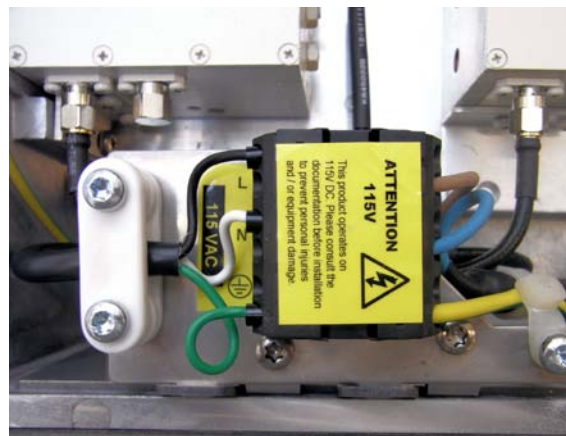
Figure 2-26: 115VAC Power Connections
