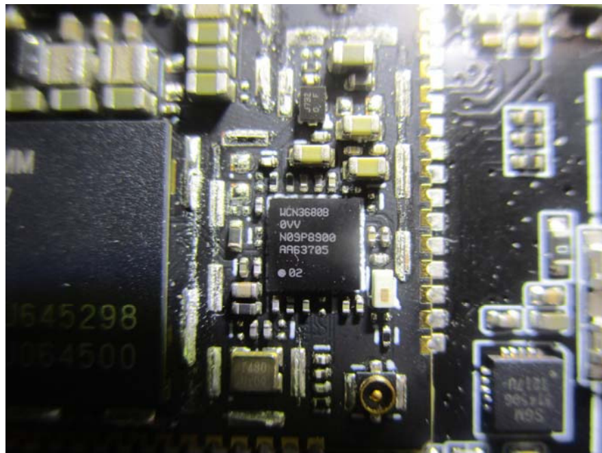
EUT – RF Chip View
