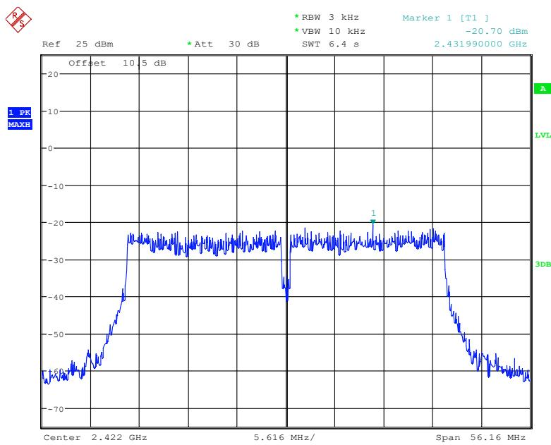
**Power Spectral Density, 802.11n-HT40 Middle Channel**
