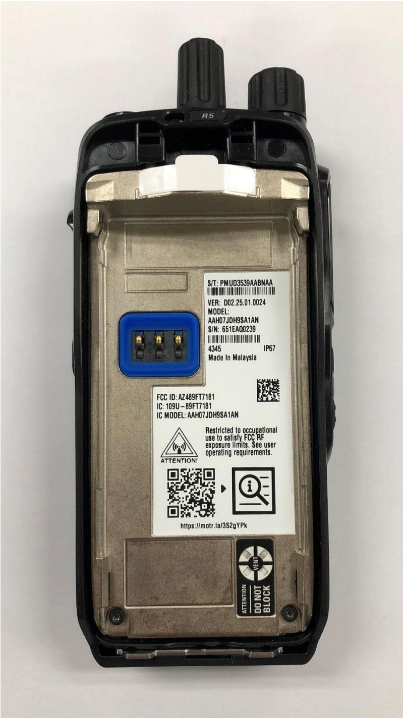
View of FCC/IC label location of Limited Keypad Model (R5)
