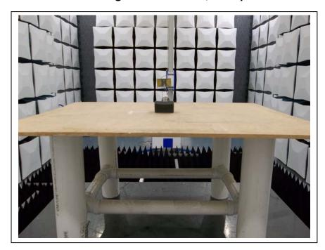
2.4 GHz: Radiated Spurious Emissions (Loop Antenna)
