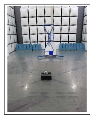
900 MHz: Radiated Spurious Emissions (Loop Antenna)
