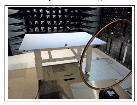
13 MHz: Radiated Spurious Emissions (Loop Antenna)
