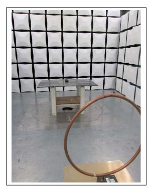
900 MHz: Radiated Spurious Emissions, Less than 1 GHz
