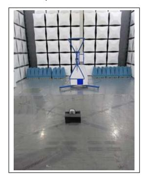
2.4 GHz: Radiated Spurious Emissions, Greater than 1 GHz
