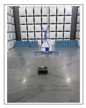
900 MHz: Radiated Spurious Emissions, Greater than 1 GHz
