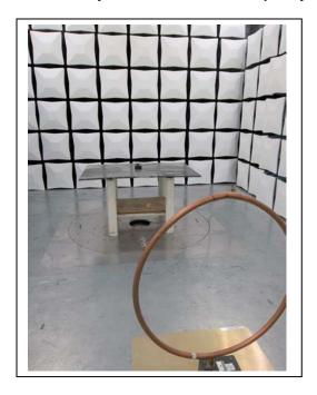
13 MHz: Radiated Spurious Emissions, 30 MHz to 1000 MHz
