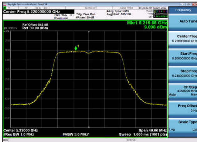
U-NII-1 Power spectral density-802.11 a(20MHz),5240MHz,Ant0
