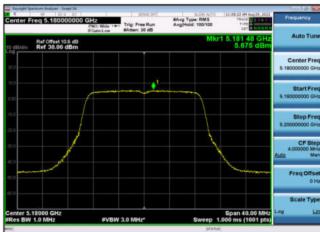
U-NII-1 Power spectral density-802.11 ac(20MHz),5180MHz,Ant0
