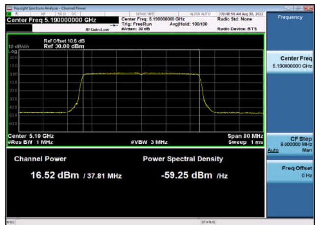
U-NII-1 Output Power-802.11ax(40MHz) ,5190MHz,Ant1
