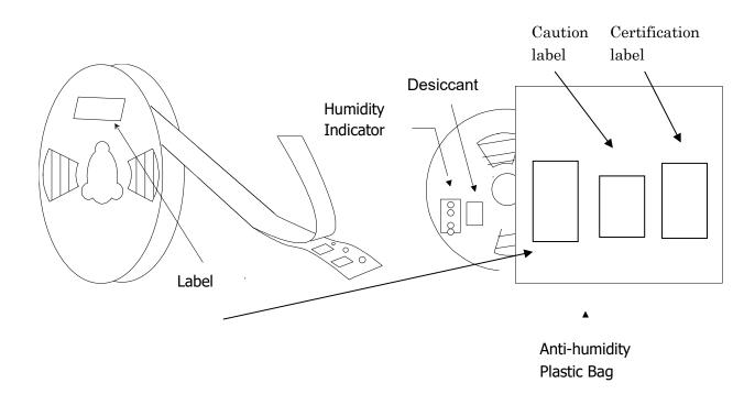
Tape and reel must be sealed with the anti-humidity plastic bag. The bag contains the desiccant and the humidity indicator.
