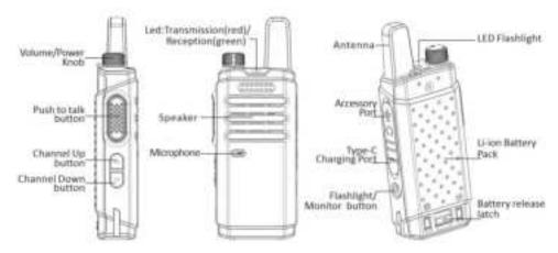
**Note:** Long press **The Flashlight/Monitoring** key to enter the monitoring state.
