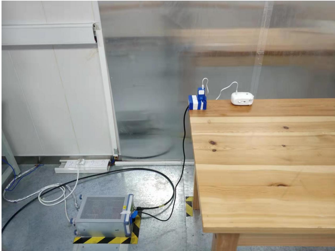
Conducted emission test setup
