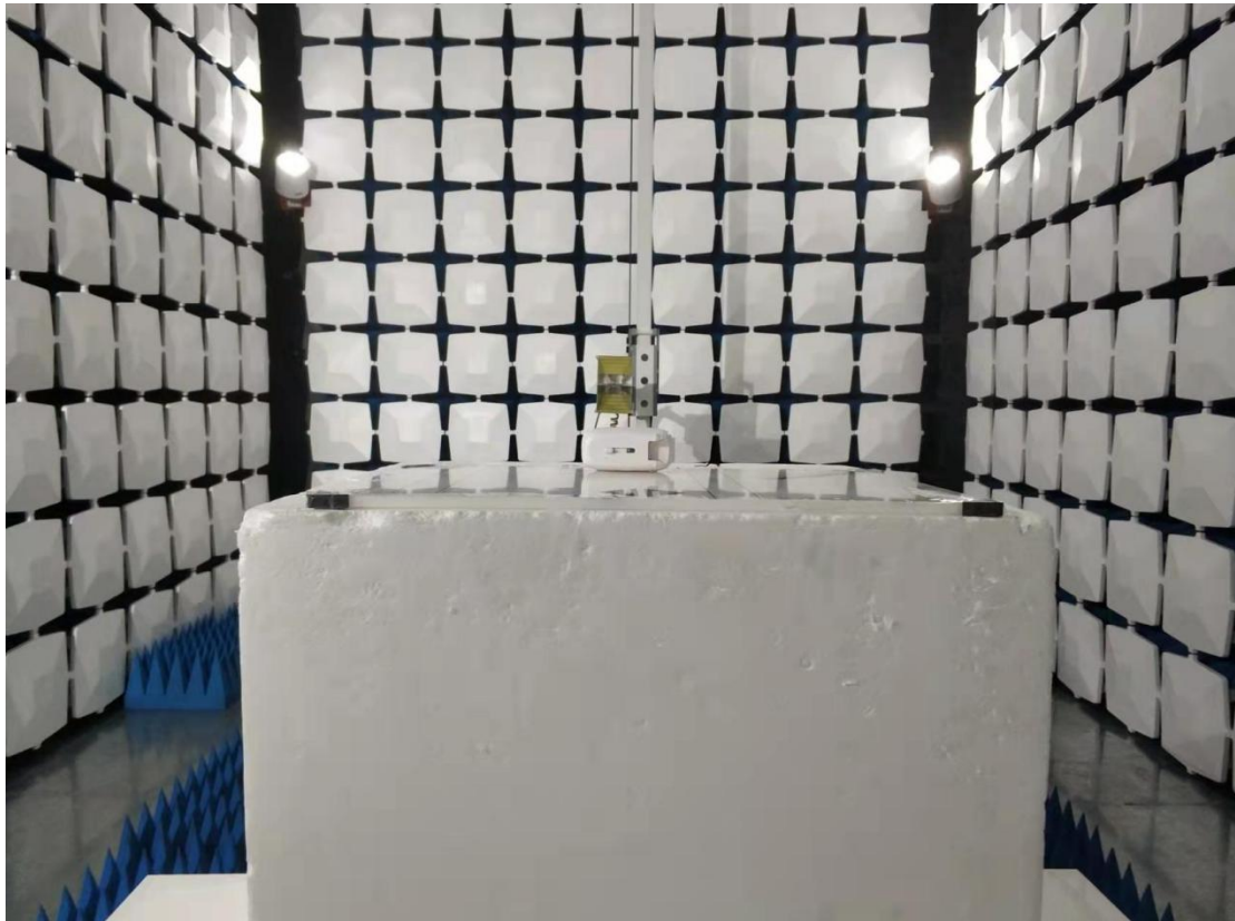
Above 1GHz for radiated emission test setup
