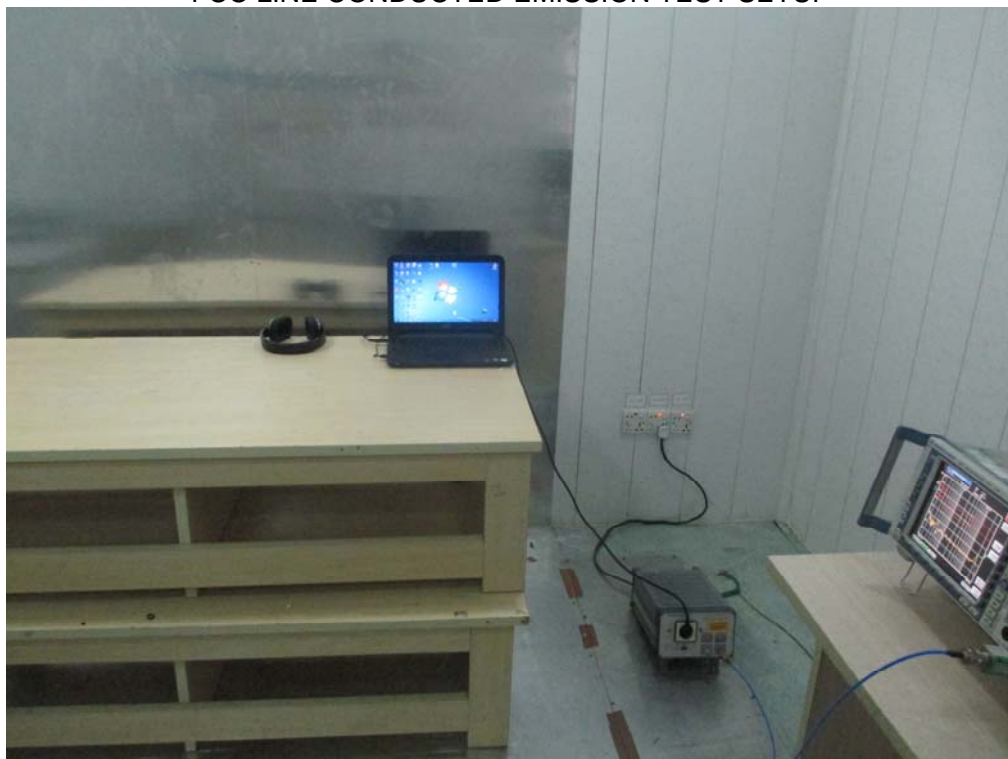
FCC RADIATED EMISSION TEST SETUP
