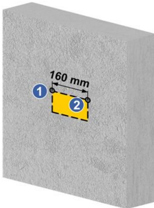
2. Drill an 80 mm-deep hole in the marked position with a  $\phi 12$  drill bit. Make sure that the hole is vertical to the wall and remove dust with a vacuum cleaner during drilling.
