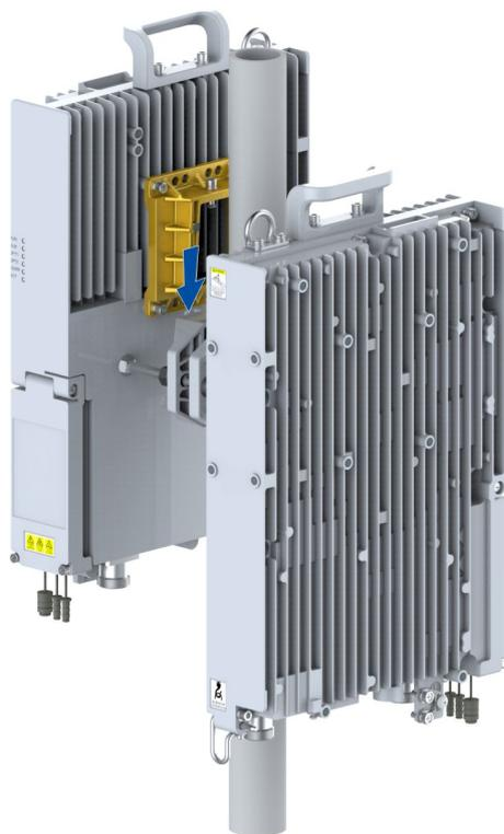
6. Tighten the captive screws on the top of all the RRU supports with an M6 Allen hex wrench respectively, see [Figure 4-27](#).
