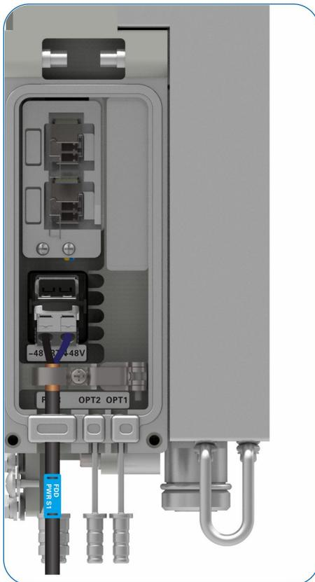
9. Use the crimping clip to crimp the naked part of the shielding layer, secure the power cable at the original waterproof plug, and ensure that the naked part has a close contact with the crimping clip.
