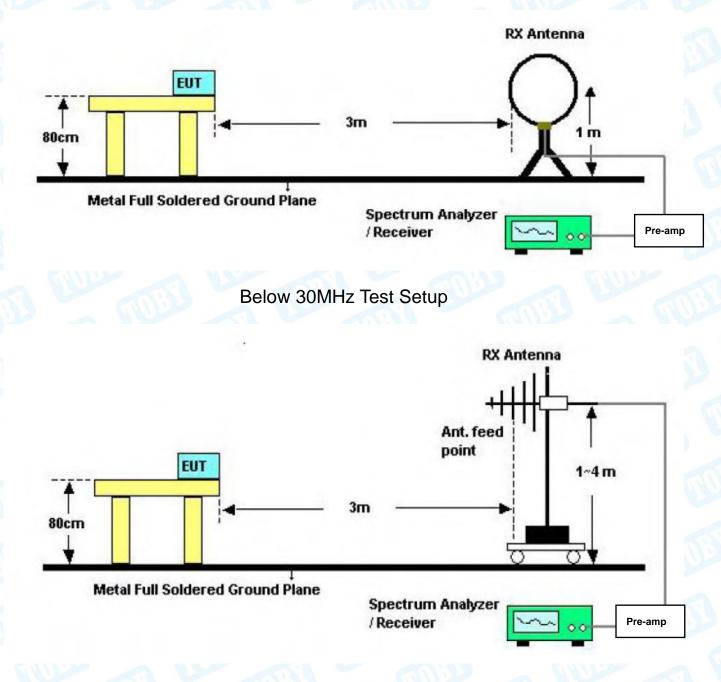
Below 1000MHz Test Setup
