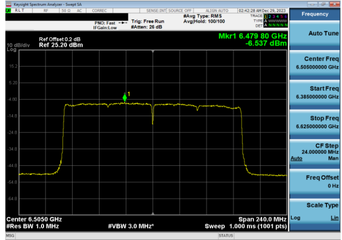
Plot 7-130. Power Spectral Density Plot Antenna WF8 Low Power Indoor (160MHz 802.11ax (UNII Band 6) – Ch. 111, MCS2)
