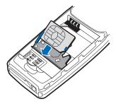
4 Swing the SIM card holder closed. The gold colored contacts on the SIM card will meet the gold colored contacts on the inside of the phone. Gently press the SIM card holder into the phone until it clicks into place.
