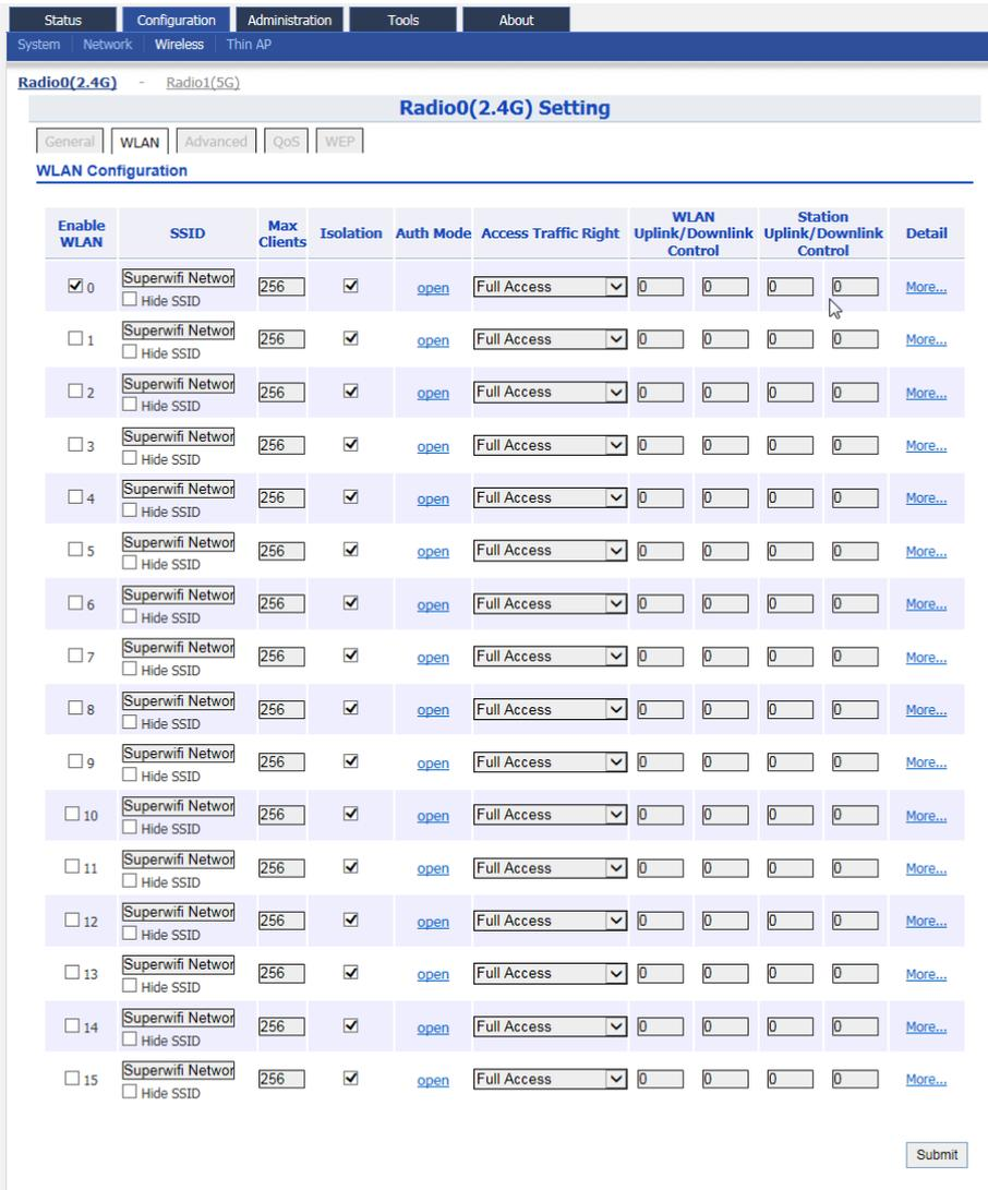
Figure 18 – WLAN List of Radio0(2.4G) of AP
