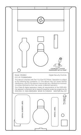
Rear housing of the unit showing placement of label (actual size)
