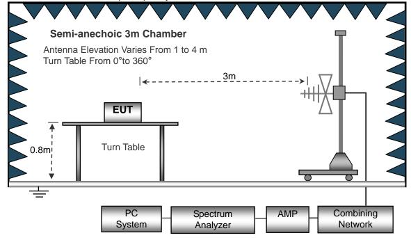
(C) Radiated Emission Test-Up Frequency Above 1GHz
