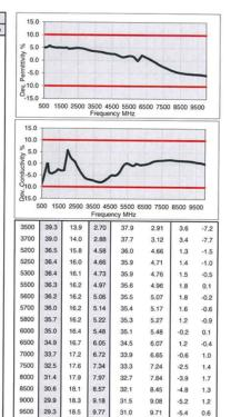
Figure B-2 600 – 5800 MHz Head Tissue Equivalent Matter
