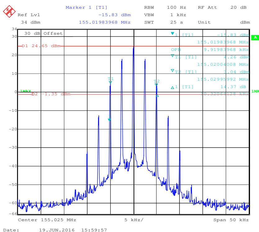
**Frequency 155.025 MHz: Emission Mask, High Power**
