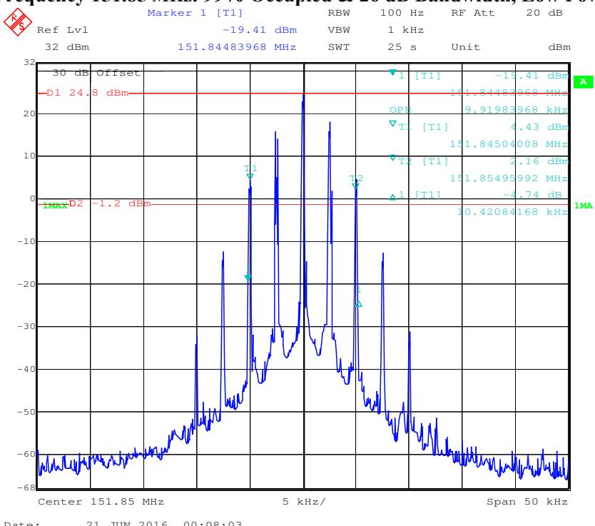
**Frequency 155.025 MHz: 99% Occupied & 26 dB Bandwidth, High Power**
