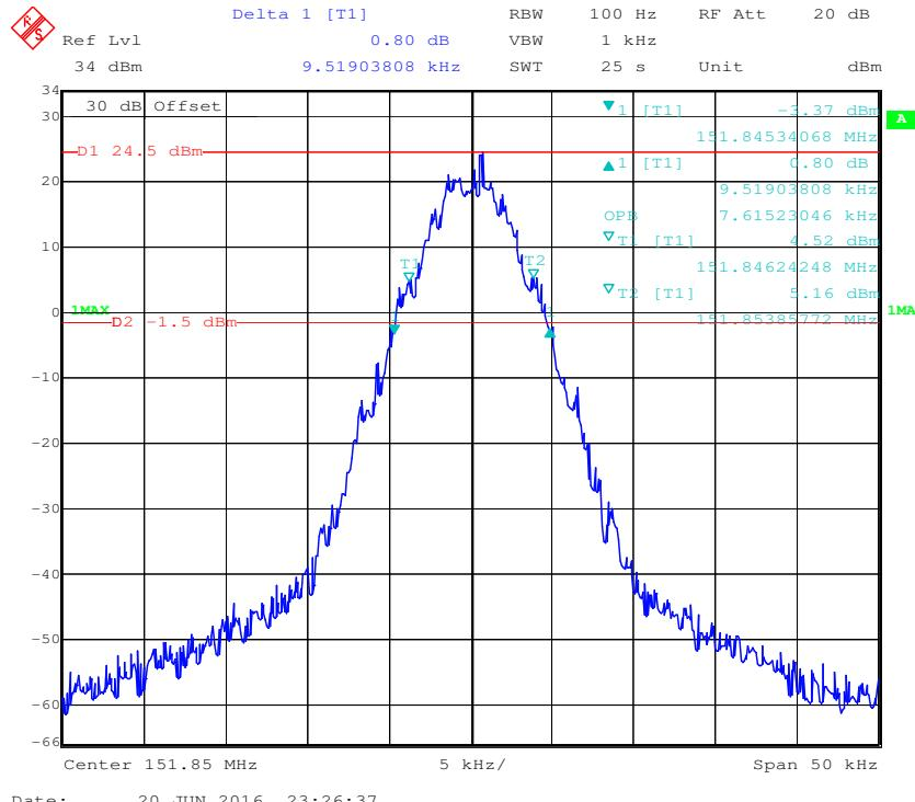
**Frequency 151.85 MHz: 99% Occupied & 26 dB Bandwidth with Low Power**
