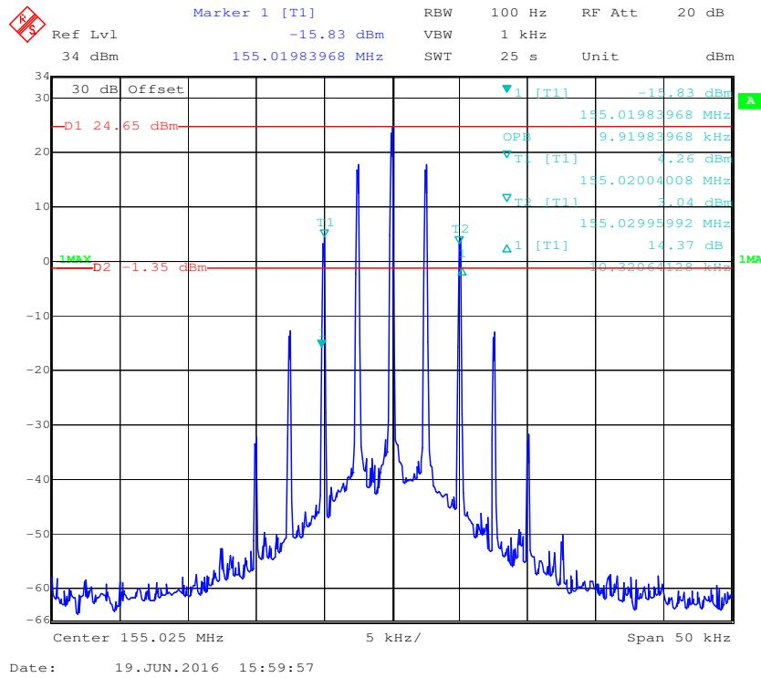
**Frequency 155.025 MHz: Emission Mask, High Power**
