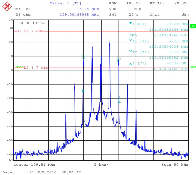
**Frequency 159.51 MHz: 99% Occupied & 26 dB Bandwidth, Low Power**
