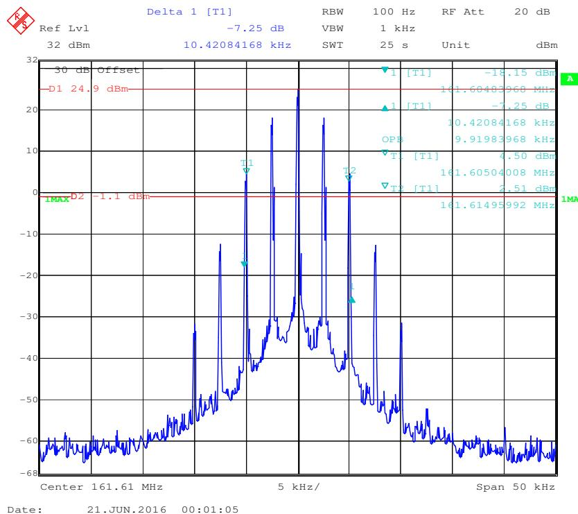
**Frequency 161.7 MHz: 99% Occupied & 26 dB Bandwidth, High Power**
