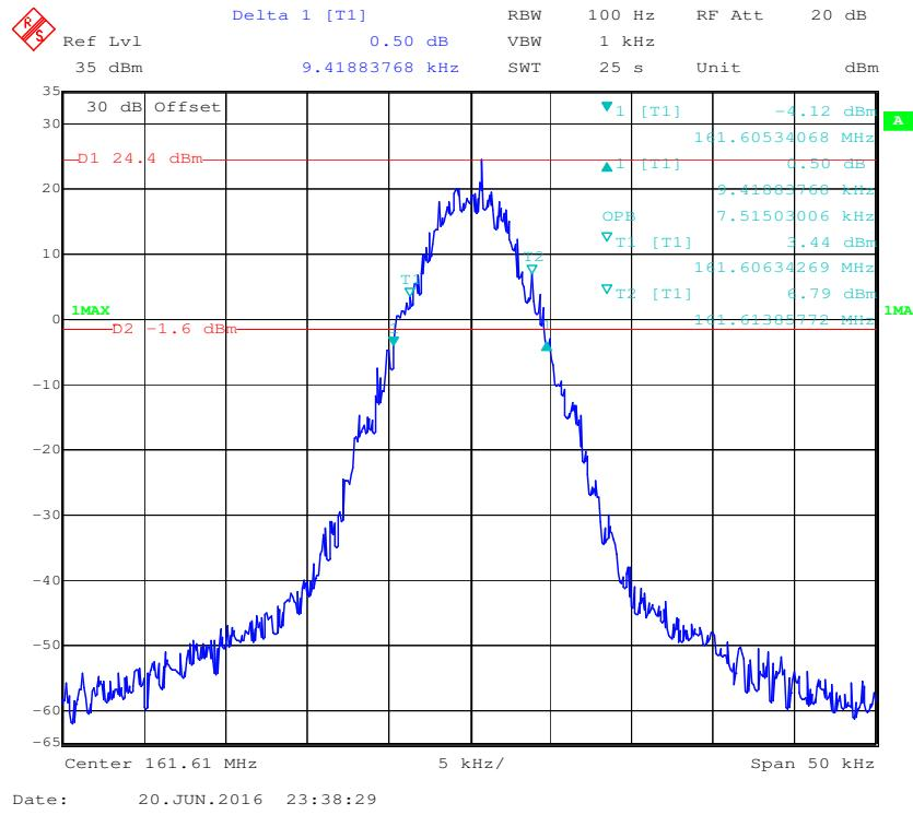
**Frequency 161.61 MHz: 99% Occupied & 26 dB Bandwidth, Low Power**
