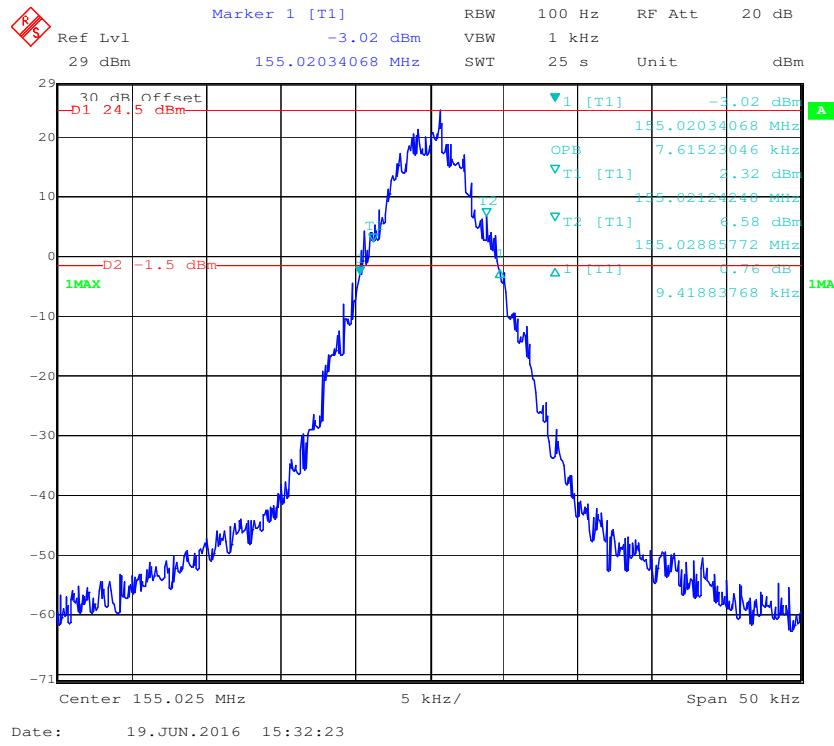
**Frequency 155.025 MHz: 99% Occupied & 26 dB Bandwidth with Low Power**
