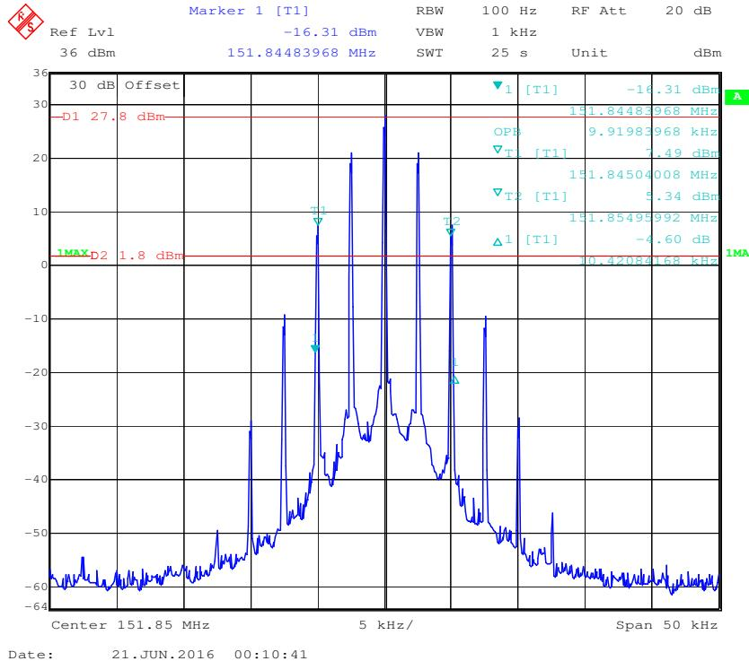
**Frequency 151.85 MHz: 99% Occupied & 26 dB Bandwidth, Low Powe**
