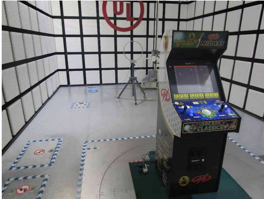
RADIATED RF MEASUREMENT SETUP (Below 30MHz)
