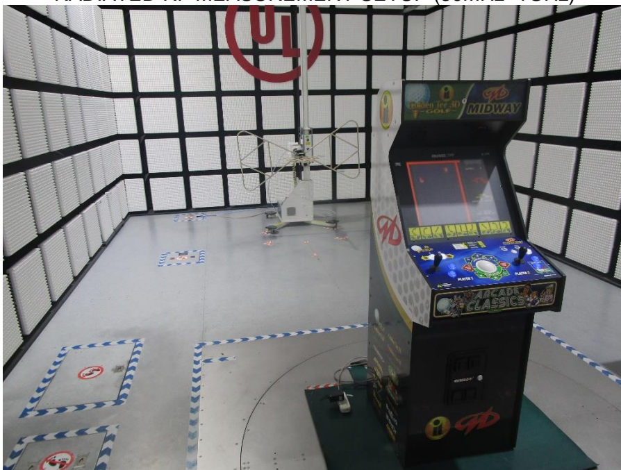
RADIATED RF MEASUREMENT SETUP (30MHz~1GHz)
