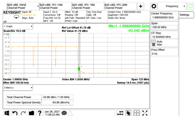
Figure 8.5-96: Conducted band edge emission at 1996 MHz, 20 MHz channel three-carrier operation (RBW = 1 MHz)
