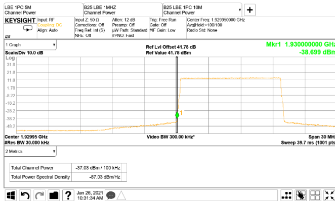
Figure 8.5-53: Conducted band edge emission at 1930 MHz, 10 MHz channel single-carrier operation (RBW = 1% of EBW)
