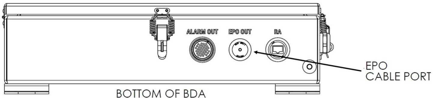
1. The EPO cable will pass into the housing and be secured with the supplied water-tight gland shown below.
