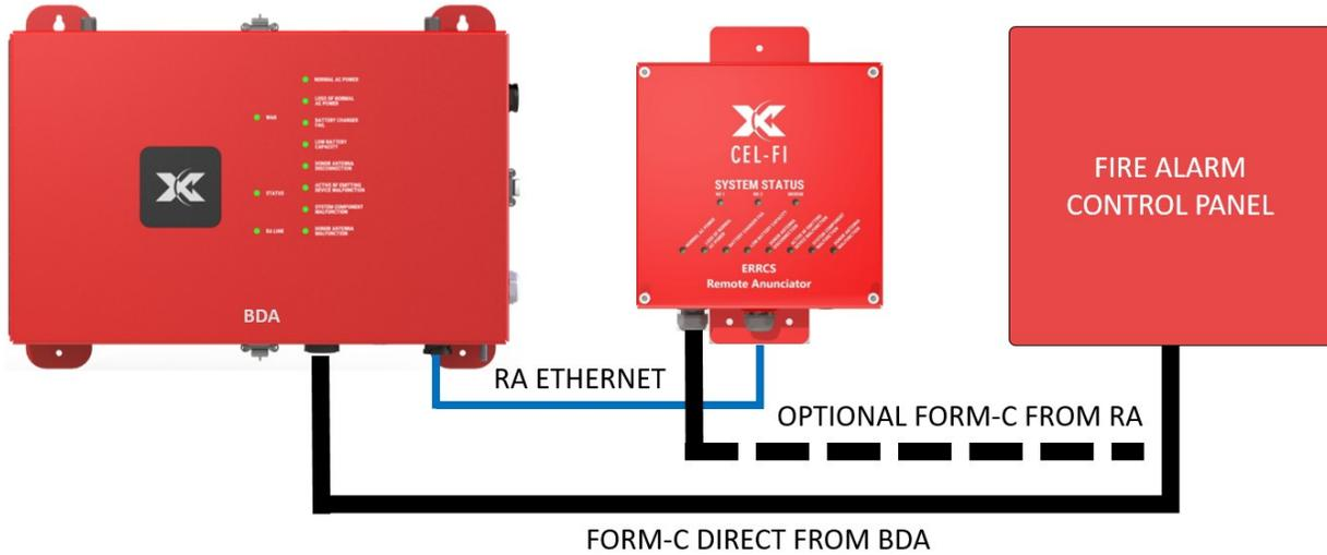
The included Form-C 24-pin cable may be used with the RA or the BDA to send alarm signals to the building Fire Alarm Panel. The cable has three pins per alarm. The first one is a normal-close signal, the second one is a common signal, and the third is a normal-open signal. Choose the appropriate signal according to the type of fire alarm control panel in the building.
