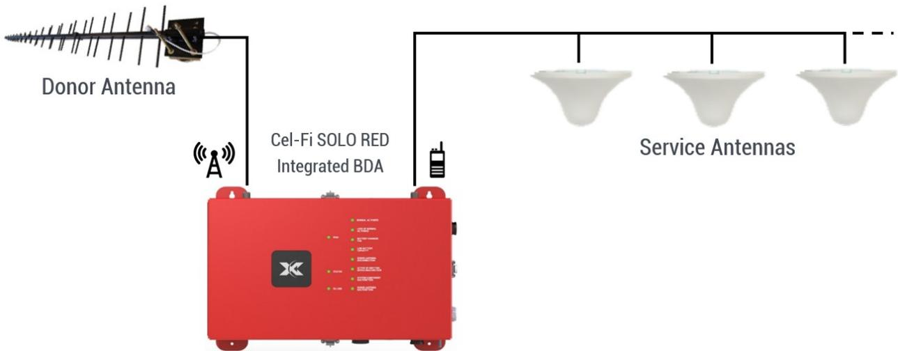
The LMR donor antenna is aimed towards the 700/800 MHz LMR High Site serving the address (GPS Lat/Long) as dictated by the AHJ or Radio Shop.
