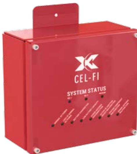
Cel-Fi's QUATRA RED Remote Annunciator Panel provides automatic supervisory signals for malfunctions of the ERRCS. It includes FORM-C dry relay contacts compatible with any fire alarm control unit (open or short circuits). The RA is connected to and powered by the Ethernet cable that connects it to the BDA.
