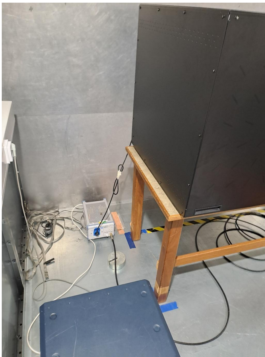
Photo 6: Photographs AC Power Line conducted emission, report section 3.3
