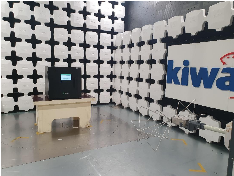
Photo 1 Photograph test setup radiated emissions 30-250 MHz, report section 3.1
