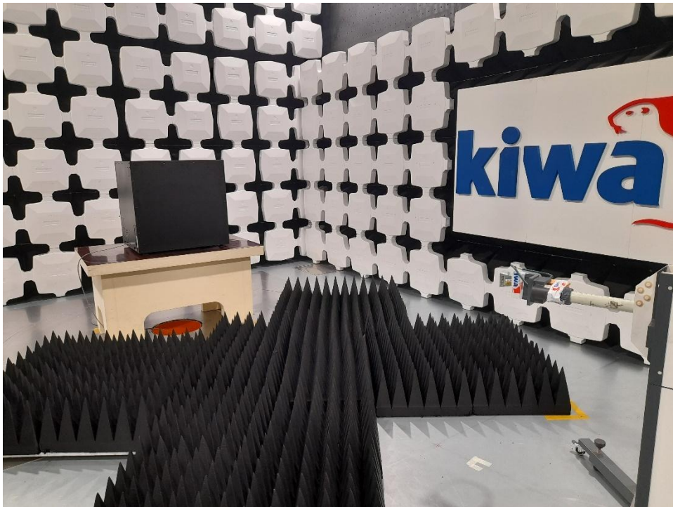
Photo 5 Photograph test setup radiated emissions 26-40 GHz, report section 3.1
